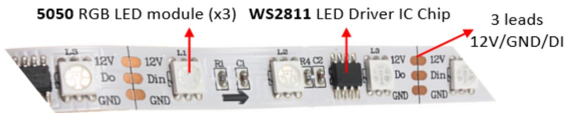
Each Segment has three 5050 RGB LED module and one WS2811 LED Driver Chip, with current limiting resistors
